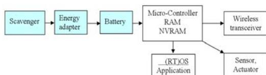
**Block diagram of environmentally powered embedded system**
