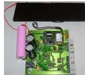
**The TinyNode wireless sensor node developed in the LCAV group at EPFL is powered up by a solar panel.**
